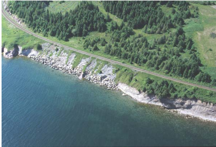
Figure 35. Aerial view of low shore cliffs composed of gypsum. Armour rock covers the rock in places to help reinforce the base of the railway line, west shore Barra Strait (Photo R. Taylor, 21 June 2001).
