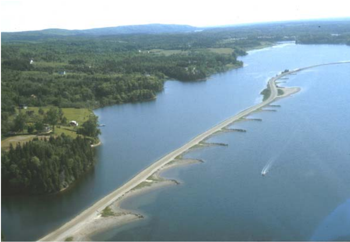
Figure 56: Aerial view of the highway at the head of East Bay where many groynes were constructed at right angles to the shoreline in an attempt to trap sediment and to protect the highway. Artificial structures decrease the ability of natural shores to respond to rising sea level by re-organizing and recycling their sediment to form new beaches. (bt260334; 25-June -1996).
